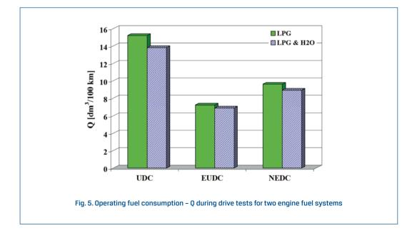
Also, additional water supply to the operating medium caused a reduction in the operating fuel consumption. Figures 6 and 7 present the relative decrease rate in specific distance emission of pollutants and operating fuel consumption due to additional supply of water to the operating medium:
