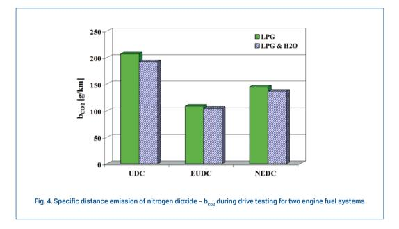
There is an evident reduction in specific distance emission of all pollutants due the additional water supply to the operating medium – varying, sometimes significantly, for particular substances and engine operating conditions. Figure 5 shows the operational fuel consumption in drive tests for two engine fuel systems.
