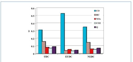
Fig. 6. The relative decrease rate in the specific distance emission of pollutants and operating fuel consumption due to additional supply of water to the operating medium
